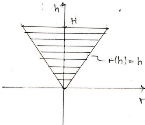
I started off by first considering the most basic top shape – a cone (Figure 9). By substituting  $r(h) = h$  and integrating the function, the moment of inertia becomes
