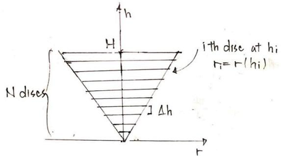
From what I have established above, the moment of inertia for one disc,  $\Delta I_i$  would then be
