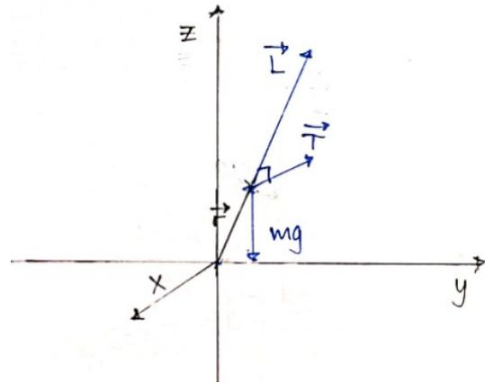
Figure 4 – Forces exerted on a spinning top
