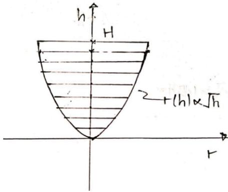
Figure 10 – top with sides  $r(h) \propto \sqrt{h}$
